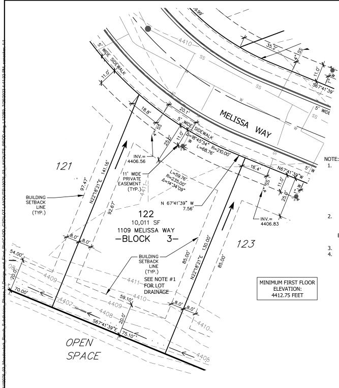
FRONT PORTION OF LOT SHALL DRAIN TO THE RIGHT OF WAY. DRAINAGE ON REAR PORTION OF LOT DOES NOT DRAIN DIRECTLY TO RIGHT OF WAY OR OPEN SPACE. THE HOME BUILDER, WITH CONSTRUCTION OF THE HOME, SHALL DIRECT OR RETAIN WATER ON
